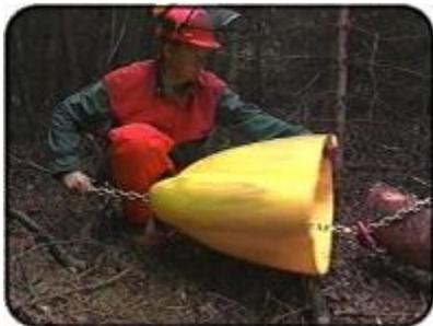
4. Set the automatic tripper on the towing rope.
