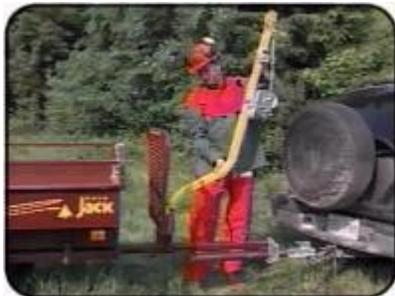
4. Attach the loading mast cable to the hook in front of the ATV trailer box.
