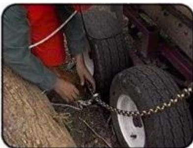
4. Operate the manual winch and the log is lifted onto the trailer. If the tension on the winch crank is too high, you can change the winch gear ratio during operation .
