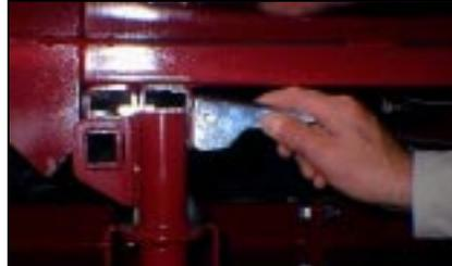
4. Position winch parallel to the metal grating for transport and attach rope to grating to secure using the winch.
