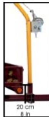
2. Install the loading mast or unloading boom parallel to the trailer.
