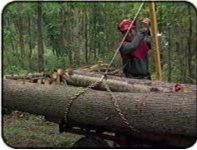
5. To unload, thread the loading mast rope under the log and connect it to the center of the V-chain.
