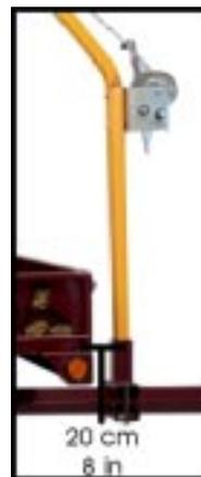
3. Install the dumpbox extension on the loading mast by lifting up the swivel pulley, sliding the boom extension over the tubing and re-inserting the swivel pulley into the tubing. Position the rope into the pulley in the front of the boom extension. (**only if you are using the loading mast as shown here**).
