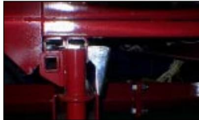
3. Next, install the loading mast (winch towards the car). The loading mast enables you to remove the box without any effort, even when you are working alone.
