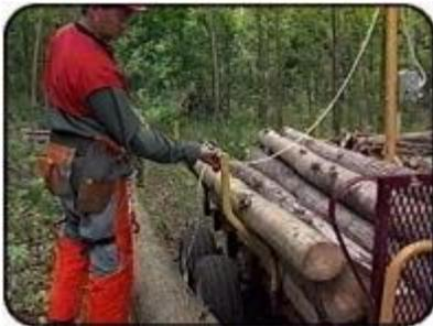
3. Next connect the loading mast rope to the center of the V-chain. Note that the rope must pass under the log before it is attached to the V-chain.
