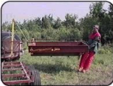
3. Position the box on the rear support and attach the latches on the front under the metal box.
