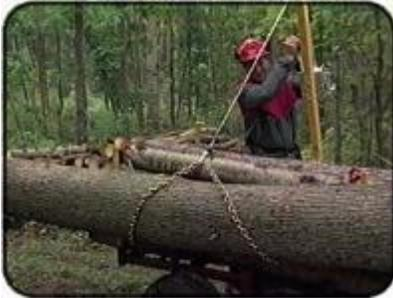
5. To unload, thread the loading mast rope under the log and connect it to the center of the V-chain.
