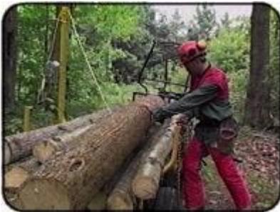
6. Turn the winch lever and the log is lifted and unloaded next to the trailer.
